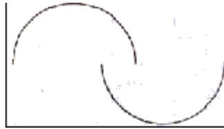
This design is also very simple, and can also be made easily from metal drums or pipe sections. The design is slightly more efficient than the one above as some of the air is deflected by the second vane as it exits the first one.
