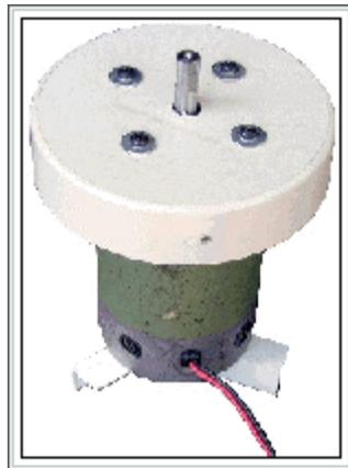
The DC motor fitted to the plastic end cap which holds it to the mast
